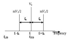
52. The antenna current of an AM transmitter is 8A when only carrier is sent. It increases to 8.93A when the carrier is modulated by a single sine wave. Find the percentage modulation.
