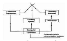
The functions of Telemetry, Tracking and Command functions are complex operations which require special ground facilities in addition to the TT&C sub system aboard the satellite.
