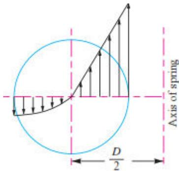
Maximum shear stress induced in the wire,
