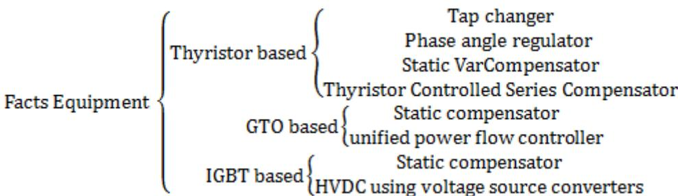
**24. Write the list of FACTS devices to control the line power flows. (MJ-14)**
