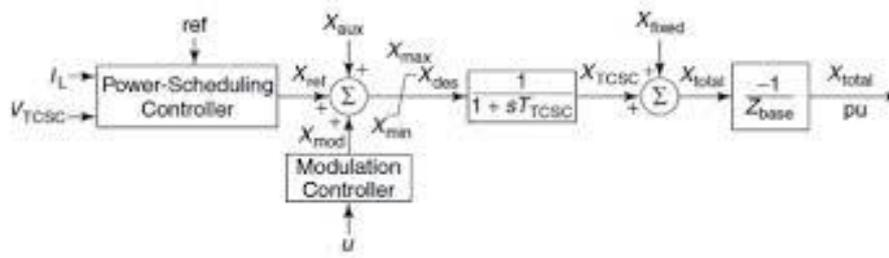
Block diagram of the variable reactance model of the TCSC
