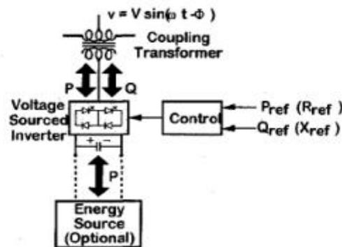
Fig. Block diagram of Stat Synchronous Series Compensator
