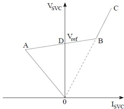
Figure : Control characteristic of SVC
