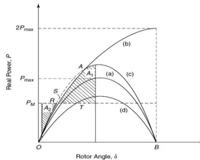
Power angle curve of SMIB system: curve (a) for uncompensated case; curve (b) with an ideal midpoint-connected SVC; curve (c) with a midpoint-connected fixed capacitor; and curve (d) with a midpoint-connected fixed inductor.
