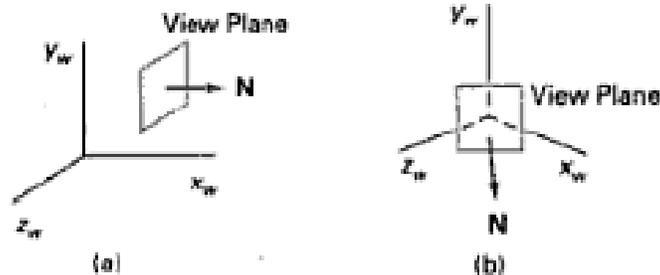
projection is 'formed' on the **view plane** (planar geometric projection) rays (projectors) projected from the **center of projection** pass through each point of the models and intersect projection plane.
